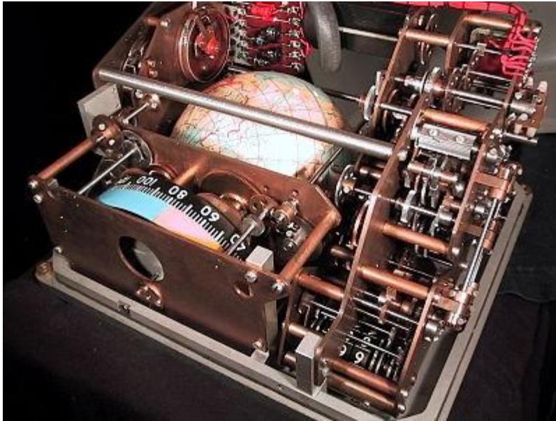
1961 - Voskhod Spacecraft "Globus" IMP navigation instrument
